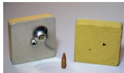
Effect of a bullet on BattleJacket coated tank – (right to left) external view, internal view
